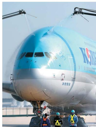
**Spring cleaning** A Korean Air A380 jumbo jet gets a wash at Incheon International Airport, Friday. It takes some 20 tons of water and 100 liters of cleaning fluid to wash the A380 plane, and around five hours to complete the task. The carrier regularly washes its planes to both make them clean and enhance their fuel economy. *Yonhap*
